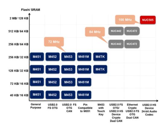
The NuMicro M451 series features ARM® Cortex®-M4 with DSP extensions and floating point unit (FPU), runs up to 72 MHz, and integrates 128/256 Kbytes embedded Flash memory, 32 Kbytes embedded SRAM, USB FS OTG, CAN and other peripherals.
